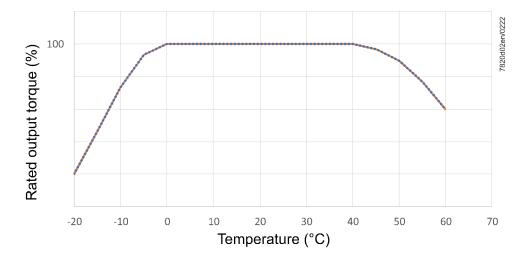
Torque under extreme/unfavorable test conditions (e.g., 100% continuous load)
