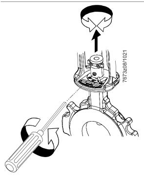
Loosen the screw. Align the coupling to suit the mounting position of the mounting plate. Tighten the screw again (max. 2 Nm).
